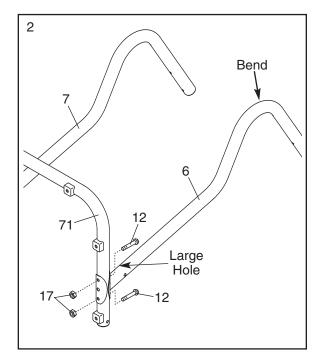
3. With the help of a second person, raise the Handrails (6, 7) so the Base (71) is flat on the floor.
